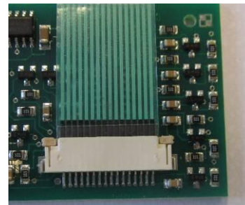
Figure 9 The other connector has contacts on the top side
