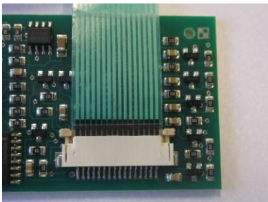
Figure 9 The other connector has contacts on the top side
