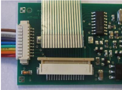
Figure 6 Foil to be inserted
